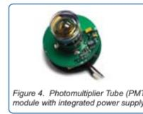
Figure 4. Photomultiplier Tube (PMT) module with integrated power supply.
