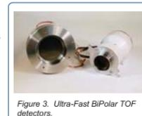
Figure 3. Ultra-Fast BiPolar TOF detectors.
