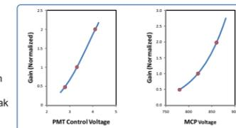
Figure 6. PMT and MCP gain as a function of applied voltage.
