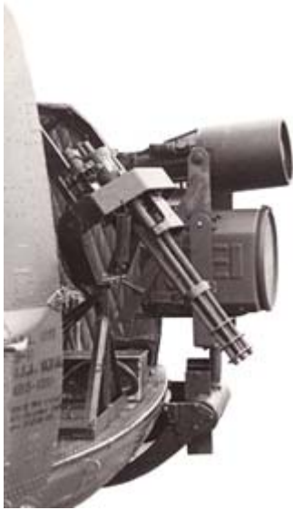
A starlight scope with external illumination aboard a Bell UH-1 "Huey" helicopter, circa 1961
