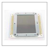
Photonis patented **ELECTROGEN™ Electron Generator Arrays (EGAs)** consist of millions of precision glass tubes fused together to produce a uniform and mechanically rigid structure. They are processed such that, when a voltage is applied across the thickness, each pore produces a beam of electrons. With each of the millions of pores producing electron, the resultant electron flux is extremely uniform and dense.
