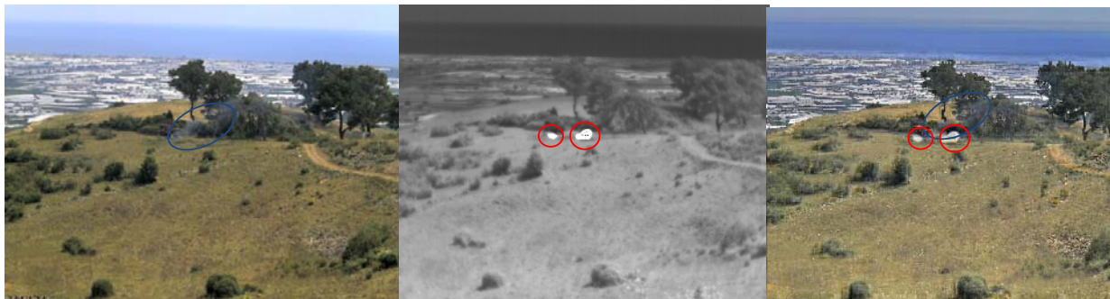
Figure 11: Iconic fusion with the visible camera (smoke) and the swir camera (fire)
