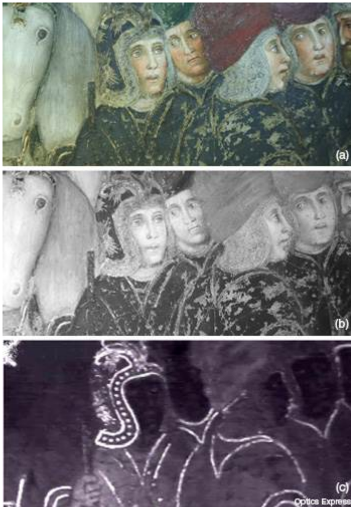
Figure 4. TQR examination carried out in the MWIR realm unveils the use of gold and silver foils in medieval wall frescos. Source: [3].
