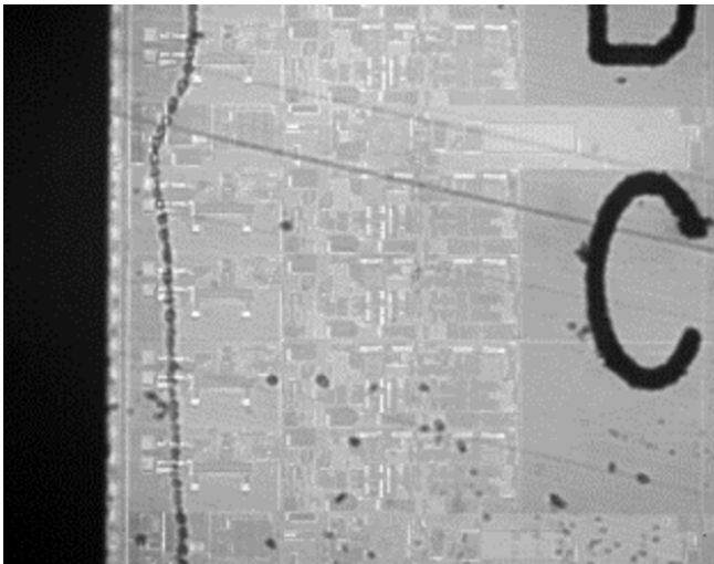
Fig. 3: Inspection of a die side – looking for dicing damage inside Si. Image taken with SWIR InGaAs camera.
