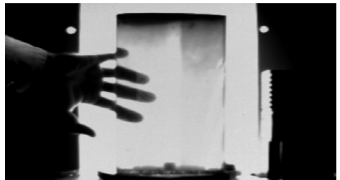
Fig. 1: SWIR InGaAs picture of a Si brick – note that the ingot is completely transparent for SWIR radiation.
