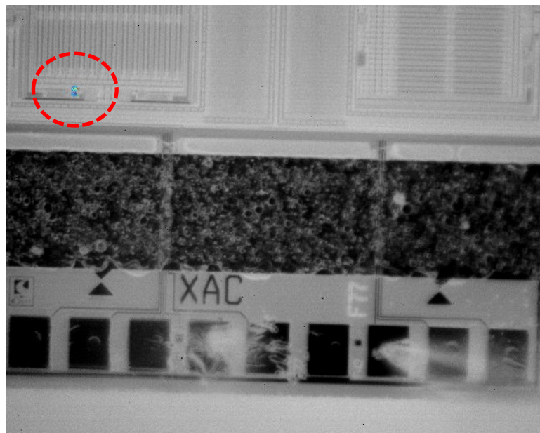
Figure 5 Overlay of thermal emission on the thermal background image. Image courtesy of SEMICAPS Pte Ltd.
