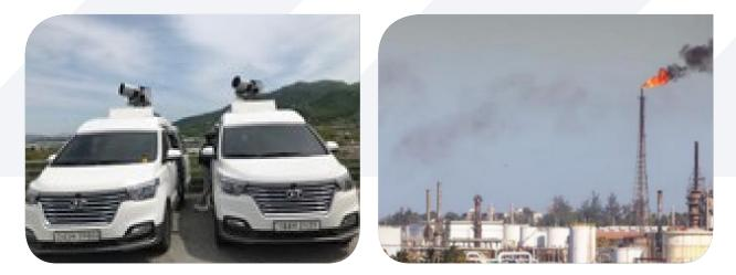
The Ministry of Environment of South Korea utilizes VSR spectroradiometers to monitor smokestack emissions as part of a national initiative to standardize and measure fugitive emissions at major industrial sites. This technology enables the quantification of the three primary greenhouse gases:  $CO_2$ ,  $CH_4$ , and  $N_2O$  enhancing environmental monitoring and regulatory efforts.
